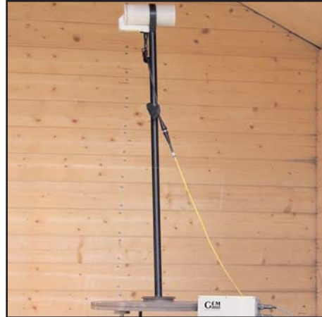
GSM-90 Overhauser Magnetometer instrumentation installed at British Geological Survey (BGS) observatory station in Eskdalemuir, South Scotland.
