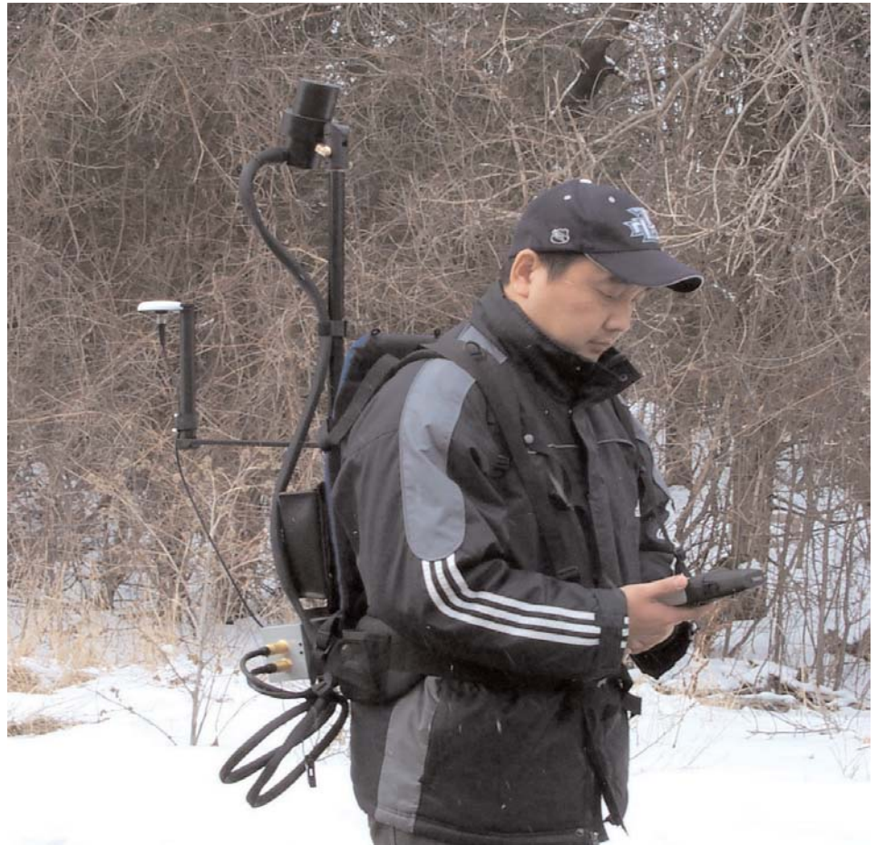
Optically pumped Potassium (GSMP-35) Resource system with Personal Digital Assistant, backpack for electronics, light weight sensors and cables.
