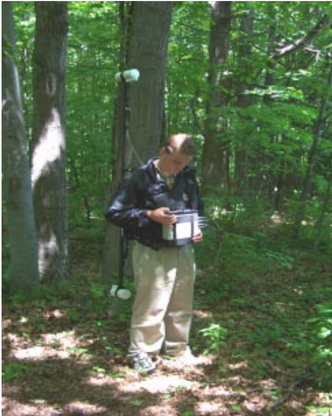
Showing the GSM-19 with backpack mounted Gradiometer
