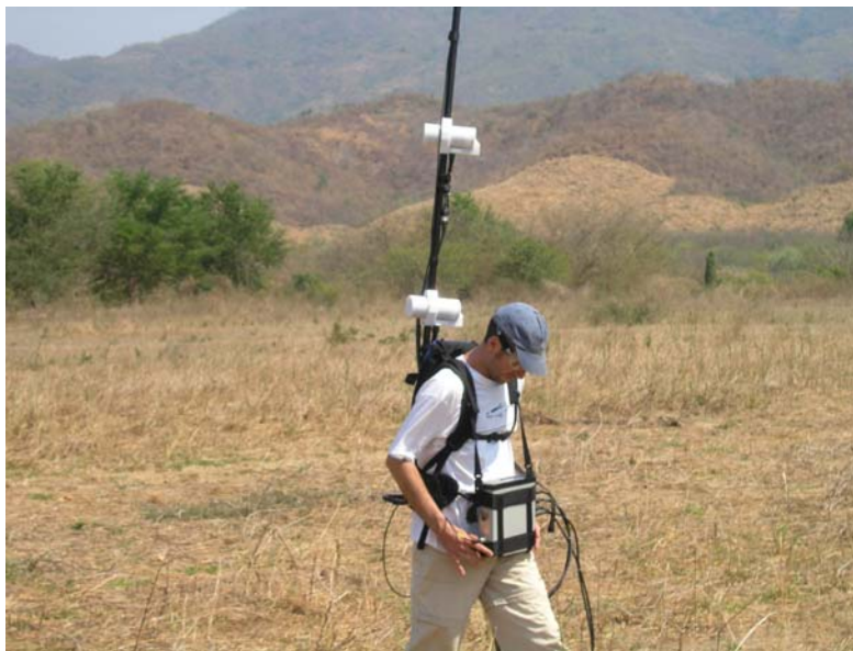
Figure 1: Overhauser quantum gradiometer with VLF attachment.
