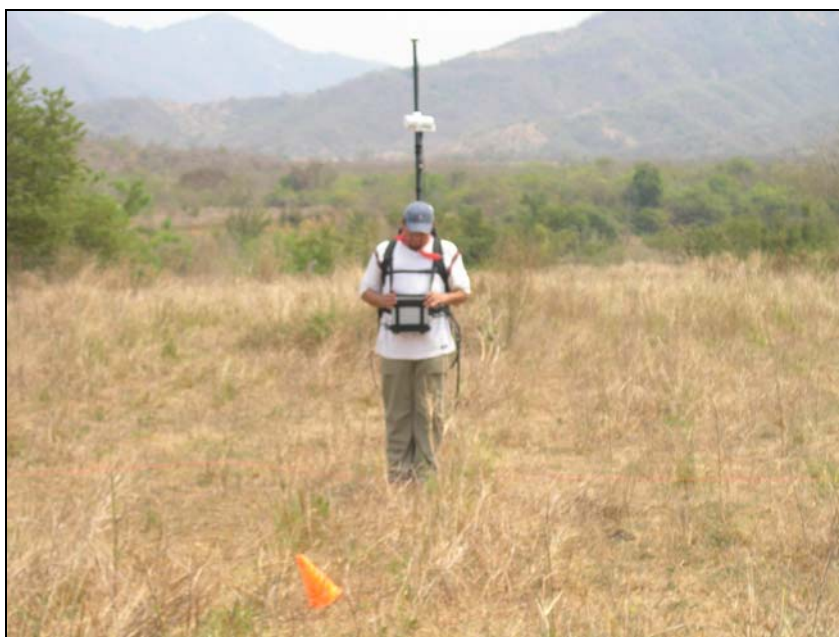
Figures 2 and 3: Acquisition of gradiometer data on site in southeastern Mexico.
