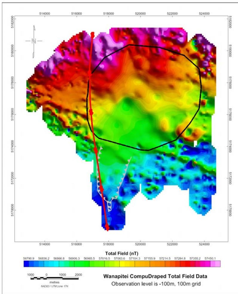
Figure 1: a) Raw Total Field data with North – South flight lines collected at 500 m line spacing and East – West tie lines collected at 2000 m line spacing, b) Microlevelled and reduced to the pole (RTP) Total Field data.
