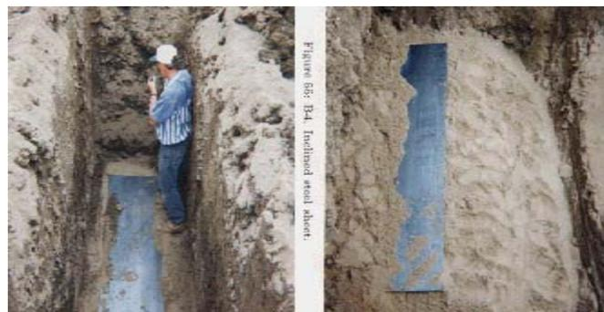
**Figure 8.** Steel plates (horizontal, dipping at 45 degrees and vertical – not shown) in Cell B4 at 2.0m depth.
