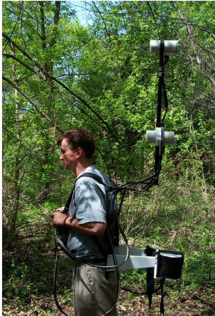
**Figure 1:** Overhauser quantum gradiometer with VLF attachment.
