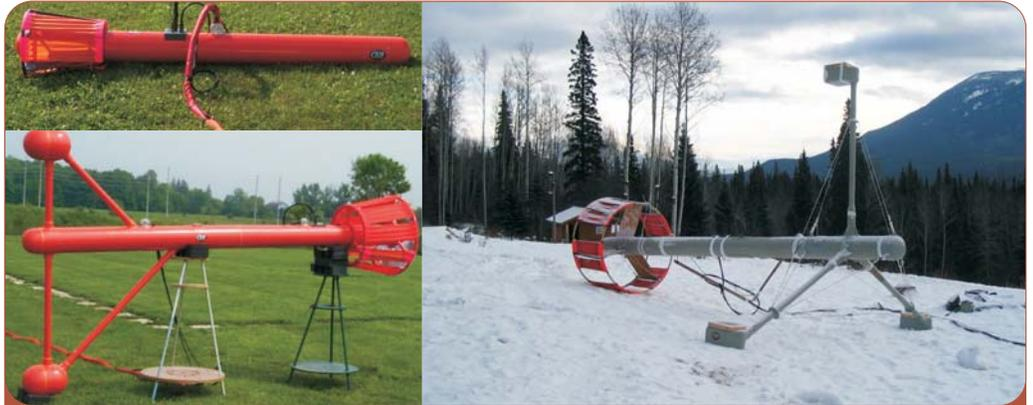
**Magnetometer, Vertical / Horizontal and Tri-Axial Gradiometers** offerings based on the latest GSMP-35A high resolution sensor.
