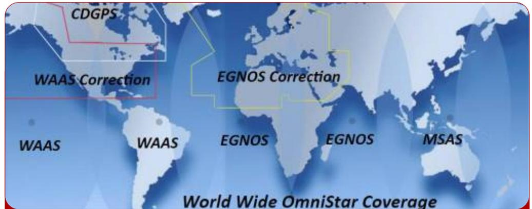
Coverage areas supported in GEM's advanced magnetometers. OmniSTAR is a global service; SBAS comprises WAAS, EGNOS and MSAS satellite systems; and CDGPS is the new Canadian standard.
