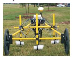
This image of a cart-borne system shows the 3D array in operation. Note that an external GPS is also provided for highly GEM's dIdD employs a mutually orthogonal coil system that measures one unbiased and four biased values of the total magnetic field. The coils are oriented to be perpendicular to the Earth's magnetic field vector, F (i.e. one coil is in the horizontal plane and one coil is in the vertical geomagnetic meridian plane).
