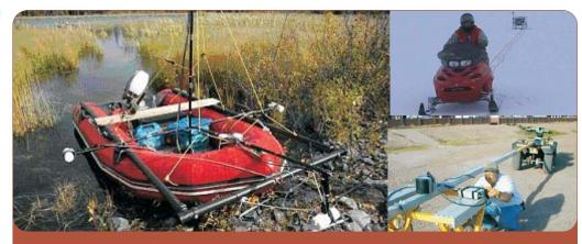
Multi-sensor configurations can be implemented on various platforms. These platforms take advantage of GEM's 4-channel "true simultaneous" capabilities
