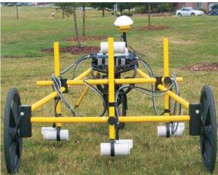
This image of a cart-borne system shows the 3D array in operation. Note that an external GPS is also provided for highly
