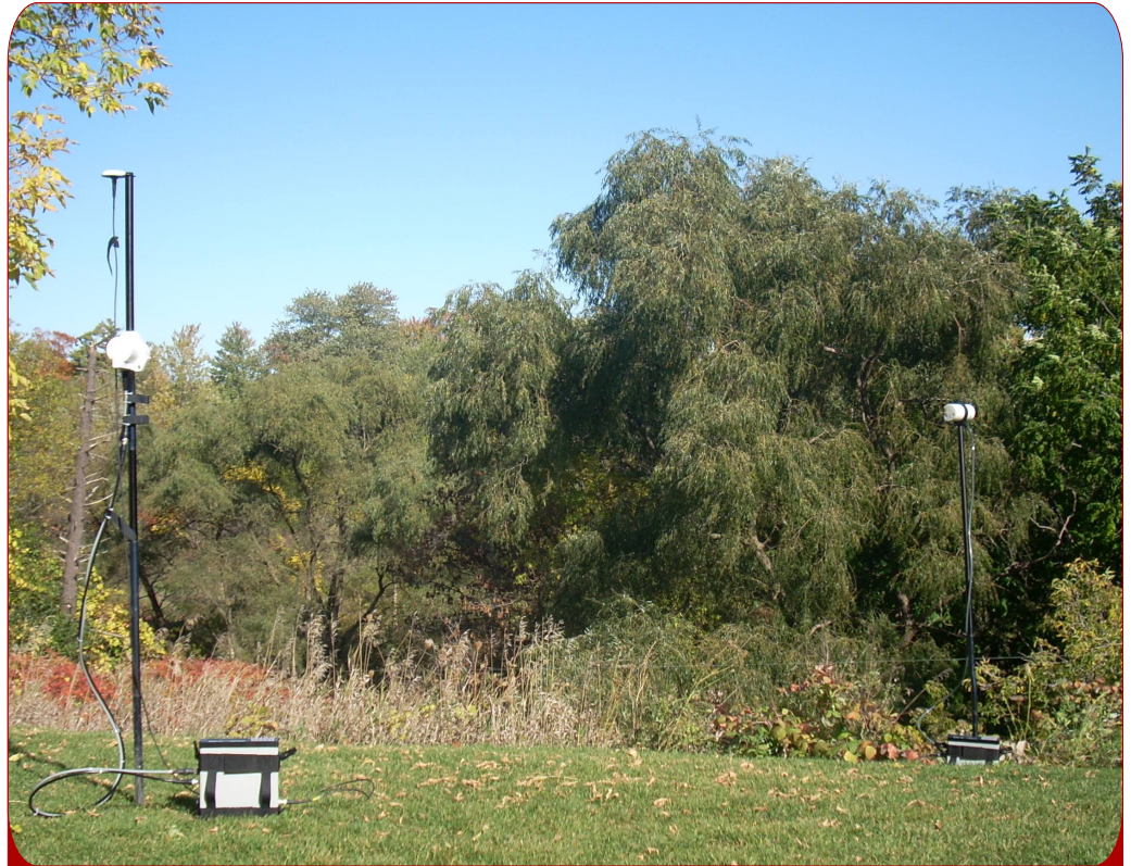
Airborne Base Station setup showing two GSM-19W magnetometers with consoles and external battery . Ground Base Station setup is similar.
