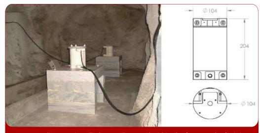
SuperGradiometer installed near Eilat, Israel within the framework of a joint Canada-Israel research project. Sensors and mounting platforms are shown.
