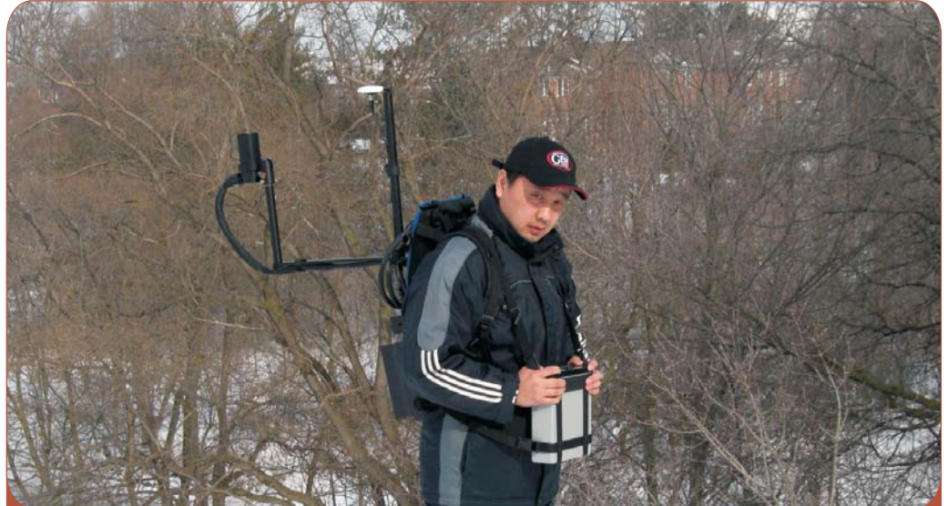
Optically pumped Potassium Magnetometer (GSMP-35 v8.0) with ruggedized console, backpack for electronics, light weight sensors and cables.
