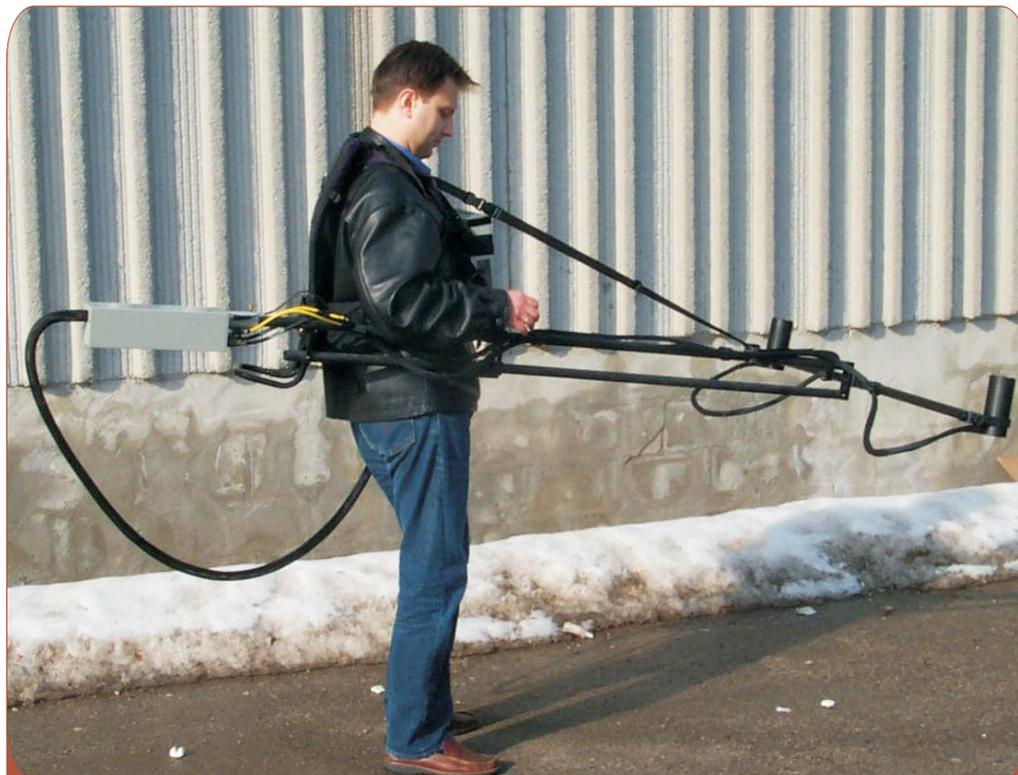
Optically Pumped Potassium (GSMP-40) ground system with electronics, light weight sensors and cable. Sensors can also be aligned vertically.
