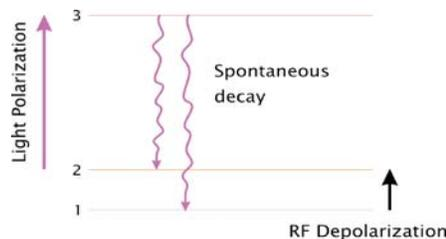
At this point, RF **de-polarization** comes into play. Here, we apply RF power of a wavelength that corresponds to the energy difference between levels 1 and 2 to move electrons from level 1 back to level 2.
