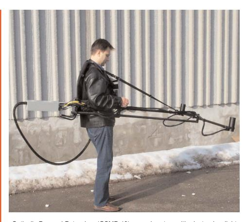
Optically Pumped Potassium (GSMP-40) ground system with electronics, light weight sensors and cable. Sensors can also be aligned vertically.
