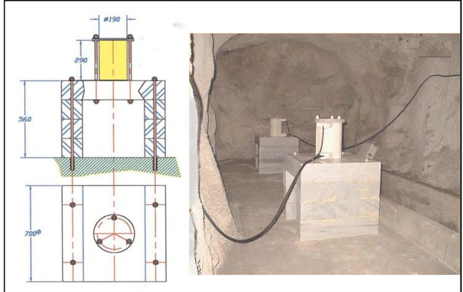
SuperGradiometer installed near Eilat, Israel within the framework of a joint Canada-Israel research project. Sensors and mounting platforms are shown.
