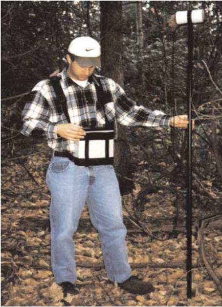
standard GEM capabilities, such as the Walking Mag option that enables the operator to sample while walking. Though there is some increase in noise, many users find this is balanced by improved field productivity. Having nearly continuous data on survey lines also helps increase the accuracy of interpretations.
