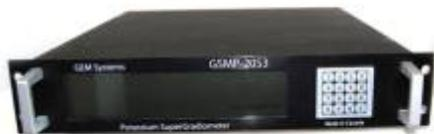
The GSMP-20S3 can achieve gradient sensitivities of 1fT/m (10-15 T/m) with a sensor spacing of 50m – a major advantage over traditional long-baseline magnetic measurements which have sensitivities on the order of 1nT.
