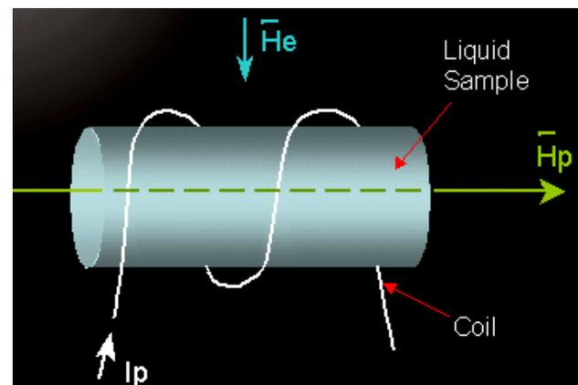
The current is then shut off and the protons precess with a frequency that is proportional to the magnetic induction. With GEM, an advanced frequency counting algorithm is used to determine
