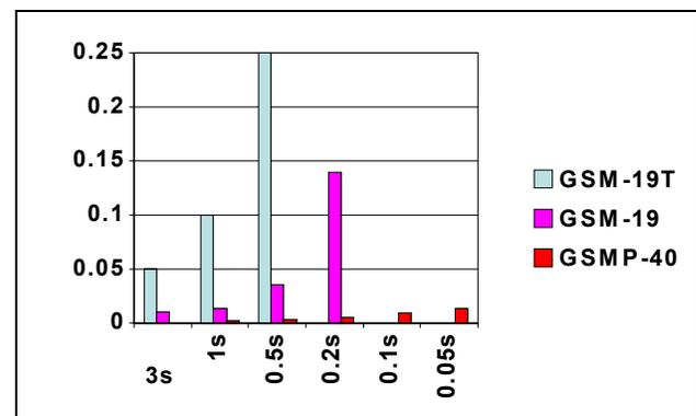
Note that the proton sensitivity at 0.5 seconds is 0.5 nT, and is cut-off at 0.25 nT for illustrative purposes.
