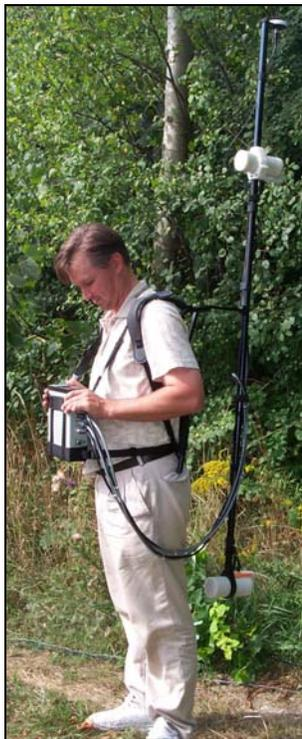
Hands-free gradiometer as required in UXO / EOD and other near surface applications. System includes built-in GPS and configurable gradiometer to eliminate diurnal effects without base station corrections.
