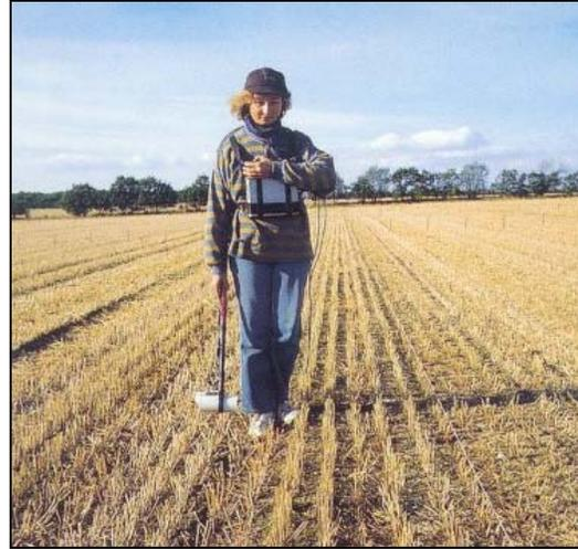
Hand-held Overhauser magnetometer applied in archeological survey application.
