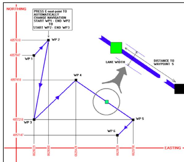
Waypoint navigation example showing path and inset with lane width. Operators navigate precisely within a pre-defined “corridor” or lane to meet exacting survey specifications.
