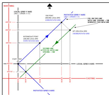
Lane rotation example showing re-orientation of paths to survey obliquely oriented targets.
