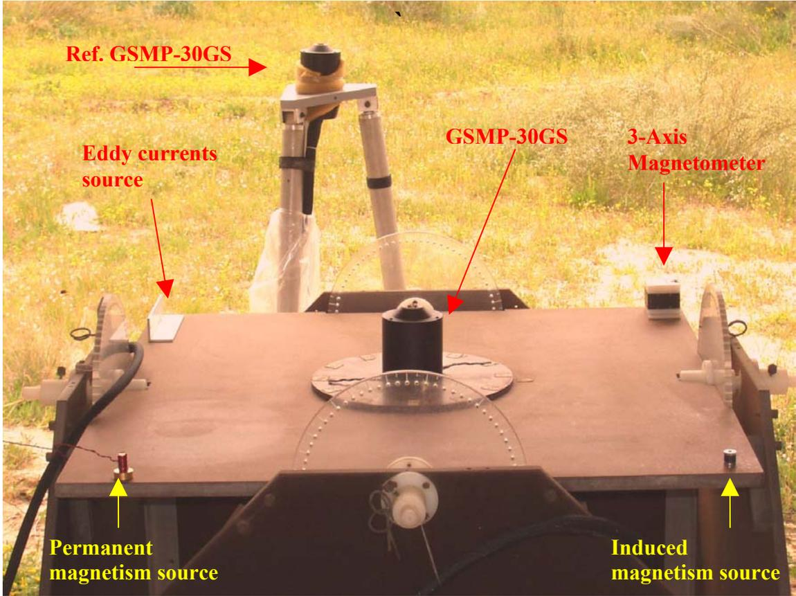
*Figure* – Picture of physical modeling with non-magnetic rotating table.
