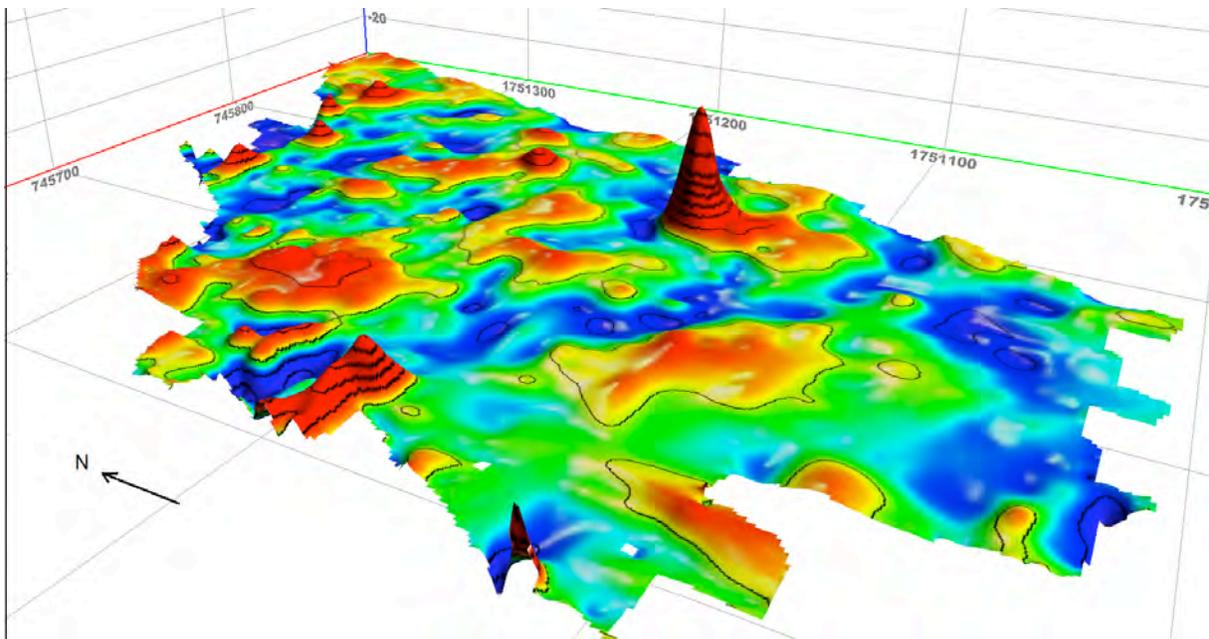
Figure 1: Site characterization map derived from Overhauser gradiometer (0.5 second sampling) for Oaxaca site. The site is characterized by a magnetically active western portion which grades into a peak anomaly to the east. The north-central and southwestern areas are quiet ... this is where monitoring sensors were placed.
