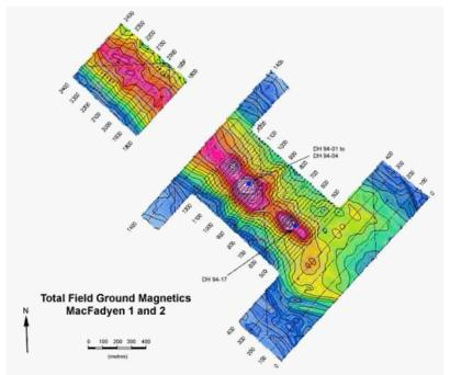
A stripping process was adopted by Scott Hogg & Associates to separate the two types of anomalies, the deep magnetic linear and the superimposed ovoid anomalies possibly representative of near surface kimberlites. The observed line profile responses were a combination of both anomaly types and as such could theoretically be separated. The spline profiles representing the magnetic response attributed to the deeper linear source were modeled with a finite length prism of variable dip,
