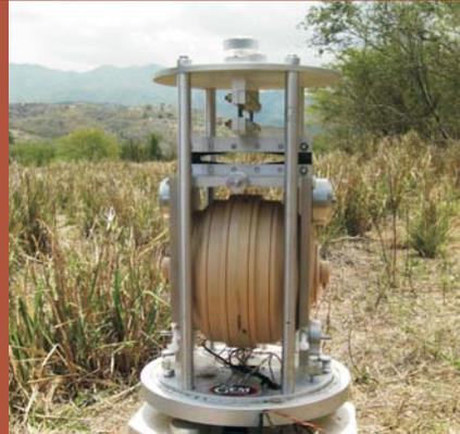
dIdD integrated 3 component coil system with enclosed Potassium sensor designed for long-term observatory monitoring applications
