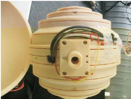
The external casing is impact resistant plastic. An upper support plate ensures that there is no movement of the sensor. The smaller sized sensor has advantages in terms of robustness (i.e. it is more durable than previous generations of larger, cylindrical sensors).
