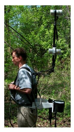
GEM's VLF system is a state-of-the-art system that enables you to acquire data simultaneously from up to 3 transmitter frequencies. Data include in-phase, out-of-phase, horizontal component (x), horizontal component (y), and field strength in pT.
