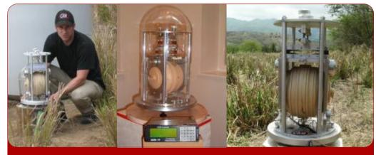
dIdD integrated 3 component coil system GSM-19FD with enclosed Overhauser sensor designed for long-term observatory monitoring applications
