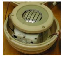
The external casing is impact resistant plastic. An upper support plate ensures that there is no movement of the sensor. The smaller sized sensor has advantages in terms of robustness (i.e. it is more durable than previous generations of larger, cylindrical sensors).
