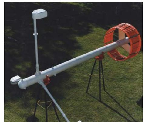
units can be installed in a special “bird” with two fins at the tips of an imaginary tetrahedron to allow for measurement of Total Magnetic Field and the gradients in three directions:
