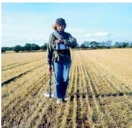
GSM-19 system in use in Denmark. This system provides a light weight, low cost solution for walking use. It also includes a "Walking" mode that enables nearly continuous coverage with resulting high productivity surveys.
