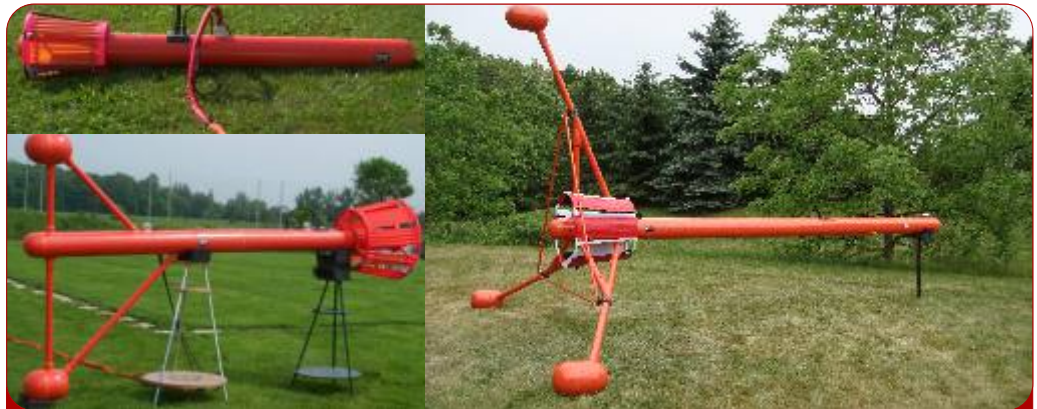
Magnetômetro GSMP-35A (B), Gradiômetro Vertical GSMP-35GA (B) e Gradiômetro Tri-Axial GSMP-35GA3 (B).
