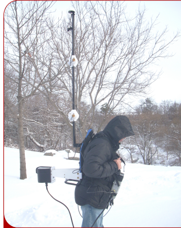
GSM-19T Proton Precession console configured with backpack, additional sensor for gradiometer (simultaneous) readings, built-in GPS and VLF EM system
