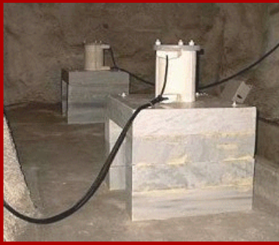
SuperGradiometer MAX installed near Eilat, geophysical laboratory Israel. Sensors and mounting platforms are shown. (<1pTesla noise level)
