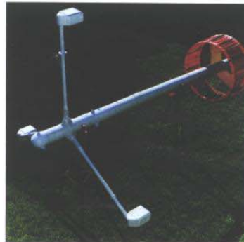
Figure 4 Airborne bird shown in fully assembled state, ready for surveying.
