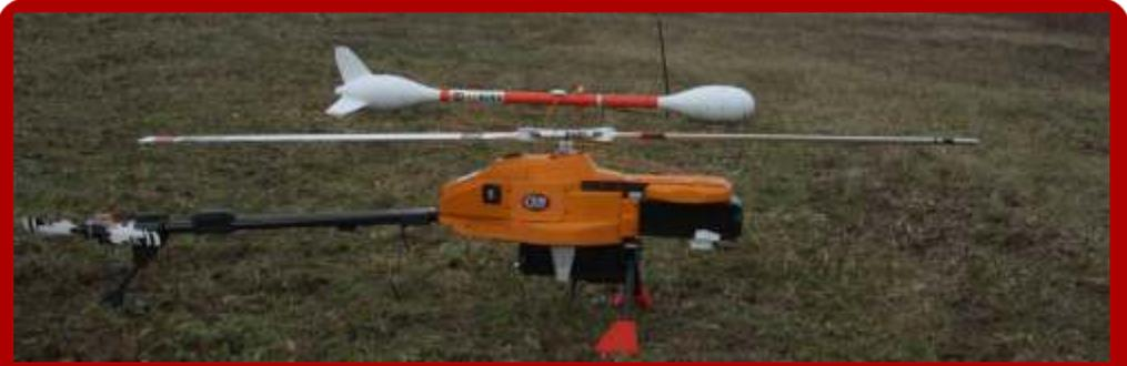
**The lightweight GEM Hawk (Helicopter) is well suited to lift the GEM AirBIRD for robust UAV aerial magnetic surveying.**
