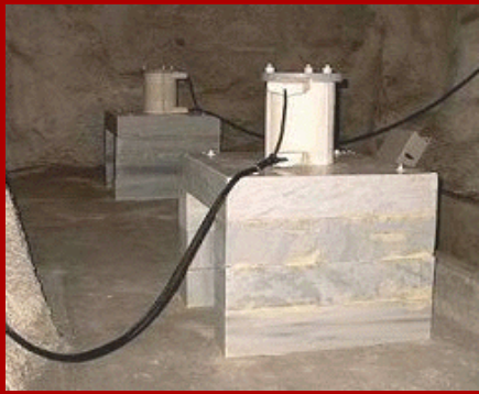
SuperGradiometer installed near Eilat, geophysical laboratory Israel. Sensors and mounting platforms are shown. (Sample data Total Field and Gradient with <1pTesla noise level)
