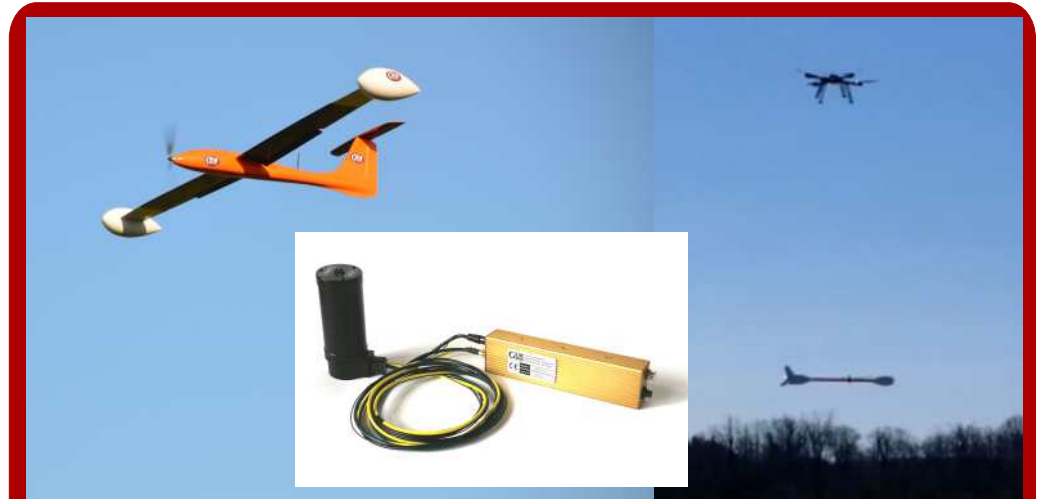
The GSMP-35U magnetometer has been installed on a multitude of unmanned platforms.
