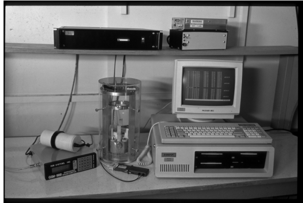
Fig. 4.5 Instruments typical of a modern magnetic observatory. Clockwise from lower right: computer for data storage and system control. Fluxgate sensor in a tilt reducing suspension; Overhauser magnetometer and sensor; fluxgate magnetometer electronics; satellite transmitter.
