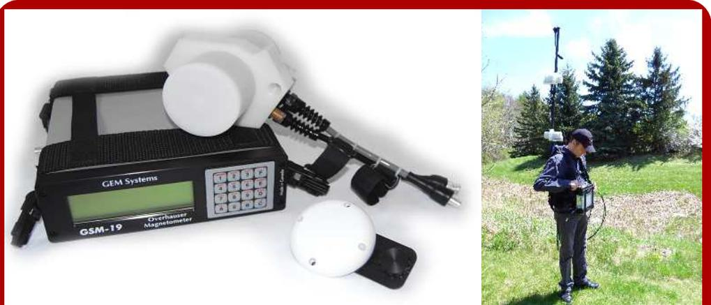
**GEM Overhauser Magnetometer system. It can be configured with an additional sensor for simultaneous gradiometer readings, walking mode, gps**
